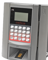
Fingerprint & Magnetic Stripe Reader
